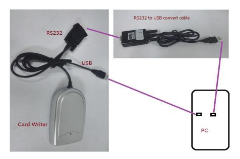
Install driver for USB-to-serial com port. (The baud rate of the card writer is 115200). Right click on the COM port and choose Properties -- Port Setting to check the baud rate.
